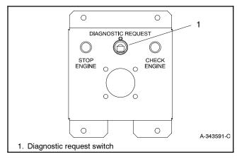
Figure 3-22 DDEC Control Box
